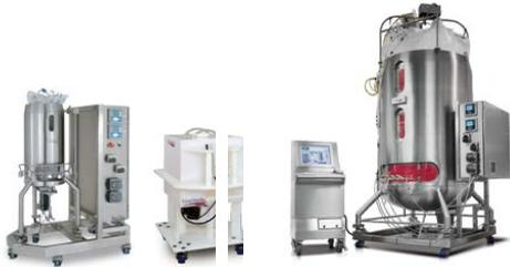
Flexible factory systems feature single-use technologies for nearly every process operation. This eliminates the expense and time required to design, construct, and validate conventional stainless steel clean-in-place/steam-in-place infrastructure. Single-use technology also provides operational savings and quality improvements by reducing cross-contamination and slashing batch-to-batch and product-to-product turnover times.
