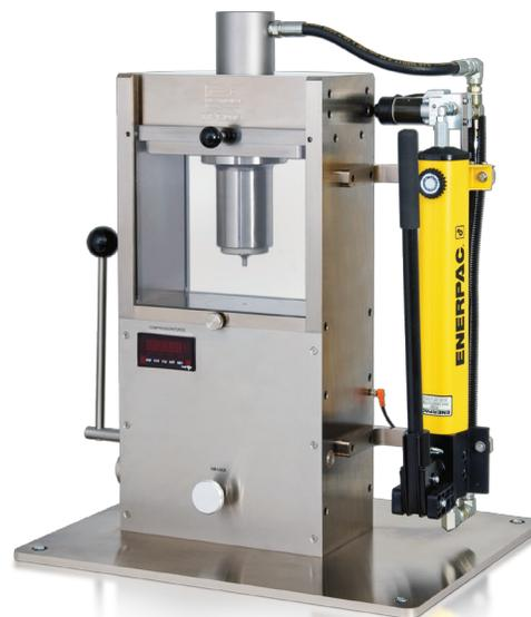
A single-station tablet press for conducting compression studies.
