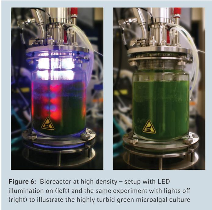
**Figure 6:** Bioreactor at high density – setup with LED illumination on (left) and the same experiment with lights off (right) to illustrate the highly turbid green microalgal culture
