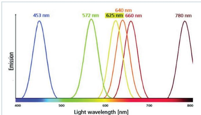
**Figure 3:** Available wavelengths of LED lights are illustrated – light spectra of the LEDs are optimized to meet various photosynthesis requirements with 453, 572, 625, 640, 660 and 780 nm available
