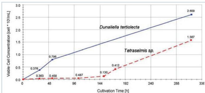
**Figure 2:** Growth of two algae strains using a DASGIP PhotoBioreactor combined with the PBR4 LED Illumination System
