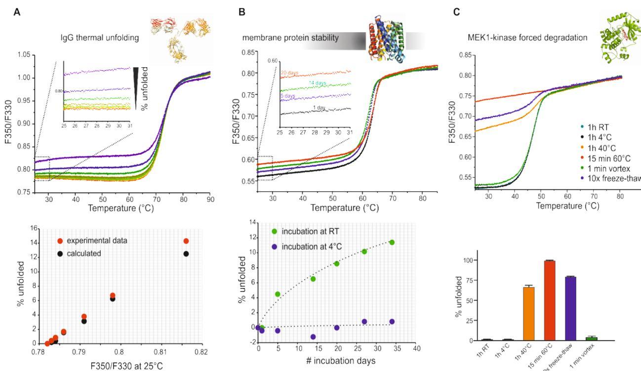
**Figure 2 A) Establishing a protein unfolding standard.** Unfolded IgG at different concentrations was mixed with folded IgG and subject to thermal unfolding. The percentage of unfolded IgG in the solution was quantified based on the F350/F330 ratio measured at 25 °C.
