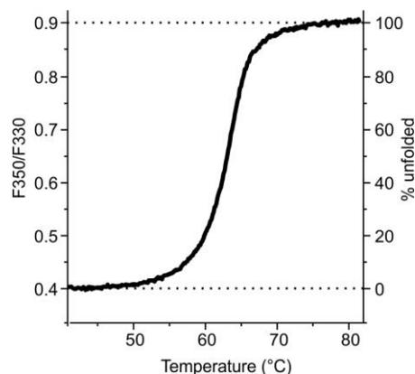
**Figure 1 Example of a typical thermal unfolding curve by nanoDSF.** The fluorescence ratio F350/F330 can be expressed as % unfolded if the fluorescence ratios of the folded and unfolded states are known.
