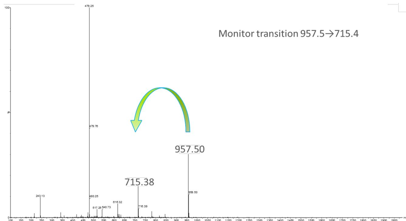
Figure 3: Waters Xevo G2 Q-TOF fragmentation data showing intact peptide and fragment ions signals selected for MRM transition monitoring
