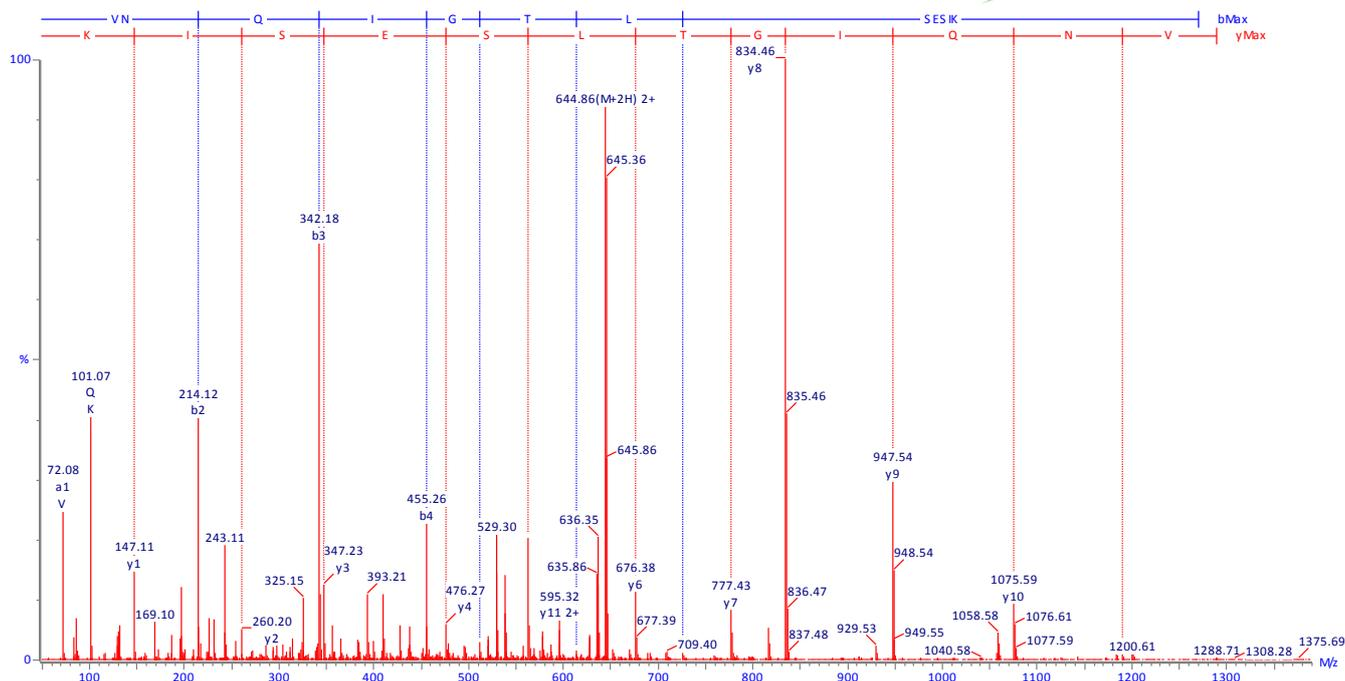
Figure 2: Automated sequence analysis of MS/MS generated fragment ions from a peptide during on-line UPLC/ES-MS analysis
