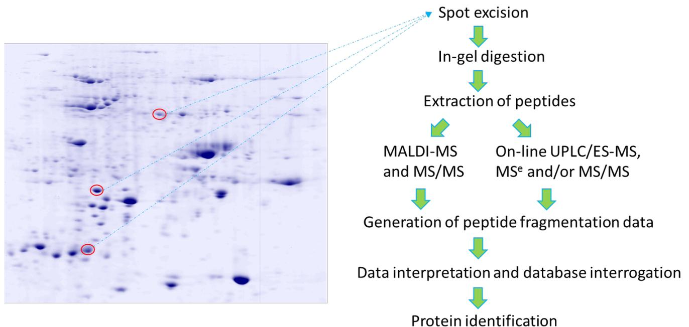
Figure 1: Phase I workflow: from 2D gel separation of a protein mixture through to protein identification
