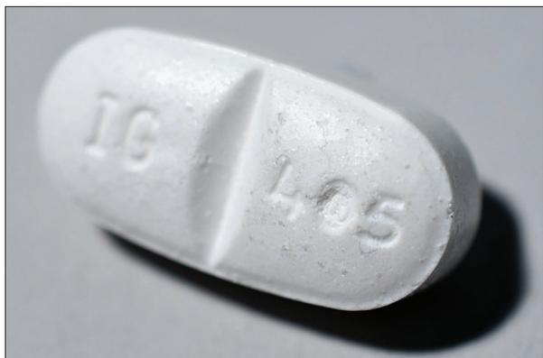
Proper setting of pre-compression requires the press mechanic to remove all pre- and main compression. Fill the press with powder and manually rotate the press while adding pre-compression force. Add this force until a tablet is ejected from the die. This tablet should look like a tablet, but fall apart when grasped. At this point the pre-compression is set and final compression added until the desired
